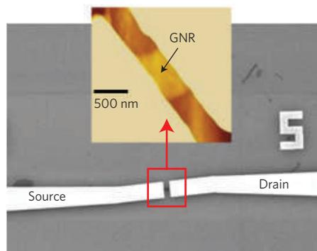
**Figure 1** | Electron microscope images of a graphene nanoribbon (GNR) that is derived by unzipping carbon nanotubes, and then connected to gold/titanium source and drain electrodes for testing in a field-effect transistor configuration. The inset shows that the nanoribbon ends are completely bonded to the electrodes. Adapted from ref. 5.
